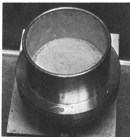
Figure 9. Americium oxalate in stainless steel filter boat
